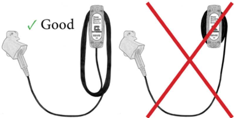
Figure 3: Drape the Charge Cable Loosely Around the PCS Enclosure.
